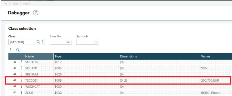
TSCCOD – use can see its type and dimensions. This shows it as an array and then the values as we have the three values from the customer.
