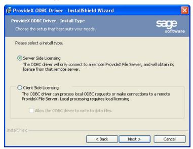
Server Side Licensing means that you are installing a *Client* version of the ODBC driver in a client-server configuration that requires access to the ProvideX File Server. *No license or activation will be requested.*
